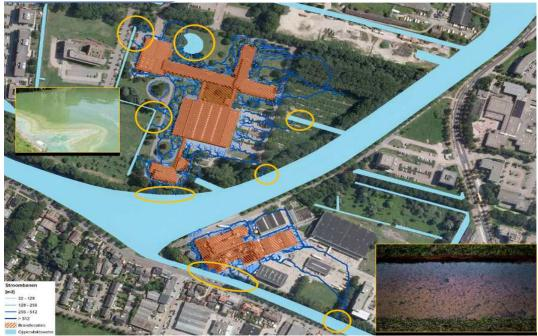
Figure 2 modelling of water with CLOUDS to prevent pollution of water and soil (The disaster resulted in 35,000 square metres of contaminated water and 1,800 tons of contaminated soil).
